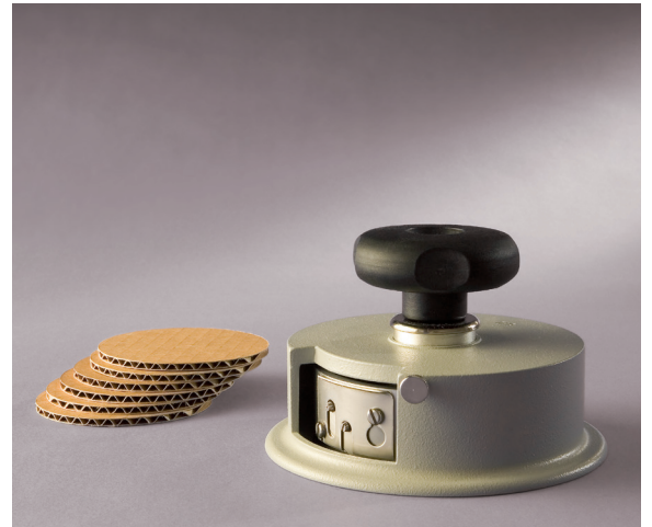
L&W Circular Cutter cuts the test pieces for FCT tests.
