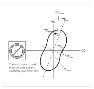
The measurement results can be presented as a polar plot, which provides a complete picture of the paper sheet's elastic properties.  $\alpha$  = TSO angle.
