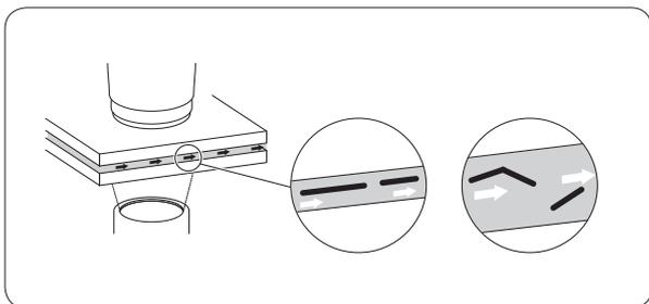
3. For measurement accuracy, a very small distance between the plates is needed. The fibres are then oriented in two dimensions, which enables L&W Fiber Tester to make a correct measurement.
