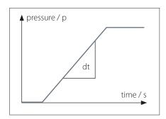
The maximum pressure change rate for mechanical pressure switches is 1,000 bar/s. For SUCO electronic pressure monitoring products the maximum pressure change rate can be up to 5,000 bar/s.
