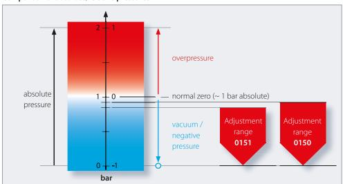
**Note:** Required set points in the vacuum range must be specified relative to atmospheric pressure (normal pressure) in the ordering process.
