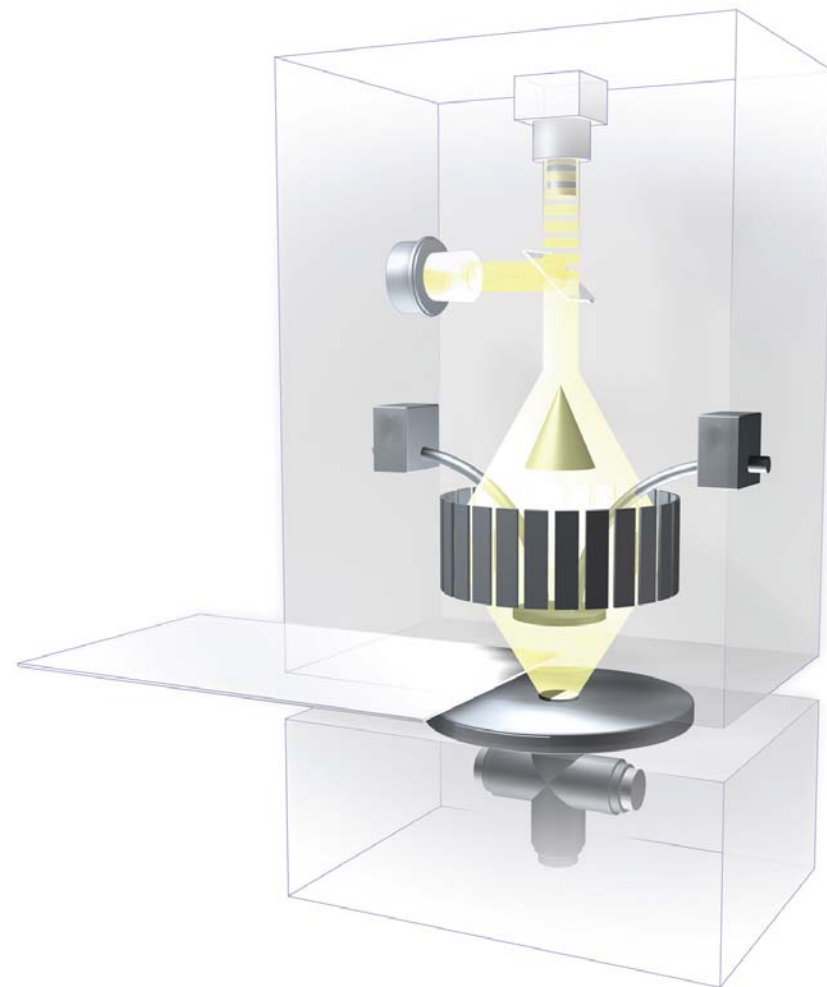
Precision Color Sensor integrates daylight and UV light sources with dual lab-grade spectrometers to measure appearance qualities online
